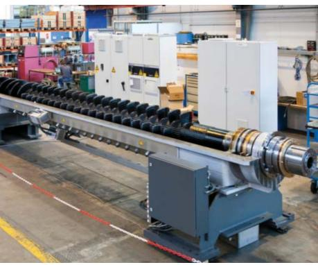
Fig 4. KX unit in the test bay at Buss AG in Pratteln, Switzerland (upper housing removed)
