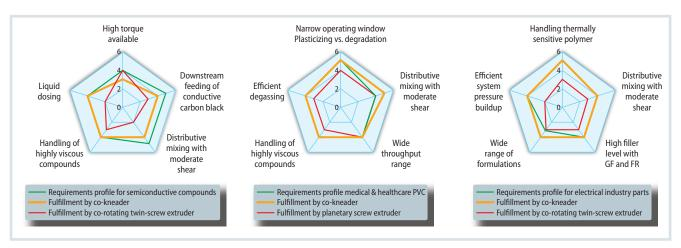
Fig. 6. Technology comparison: degree of fulfillment of requirements for manufacturing a) semiconductive compounds for high-voltage cables, b) PVC compounds for medical technology, and c) parts for the electrical industry, each in comparison with a competing compounding technology; GF = glass fibers, FR = flame retardants [5] Source: Buss; graphic: © Hanser
