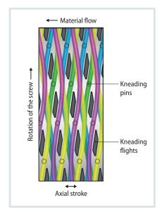
Fig. 5. Mixing effect of a four-flight screw element spread out in the plane and abstractly represented using the kneading pin paths that arise during one complete revolution of the screw shaft. The plastic mass is sheared, split, and refolded between the kneading pins and the kneader flights passing them in real operation. Source: Buss; graphic: © Hanser
