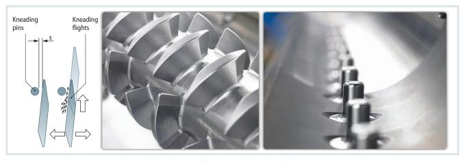
Fig. 3. In operation, the plastic mass is sheared in the shear gap (left) between the kneading flights (center) and kneading pins (right) [4] Source: Buss; graphic: © Hanser
