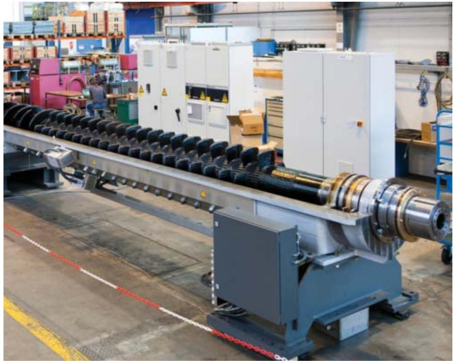
Fig 4. KX unit in the test bay at Buss AG in Pratteln, Switzerland (upper housing removed)
