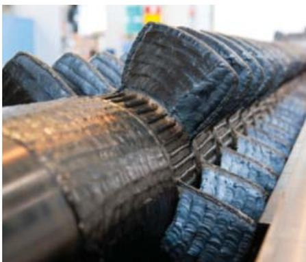
Fig 2. Close-up picture of armoured 4-flight screw design
