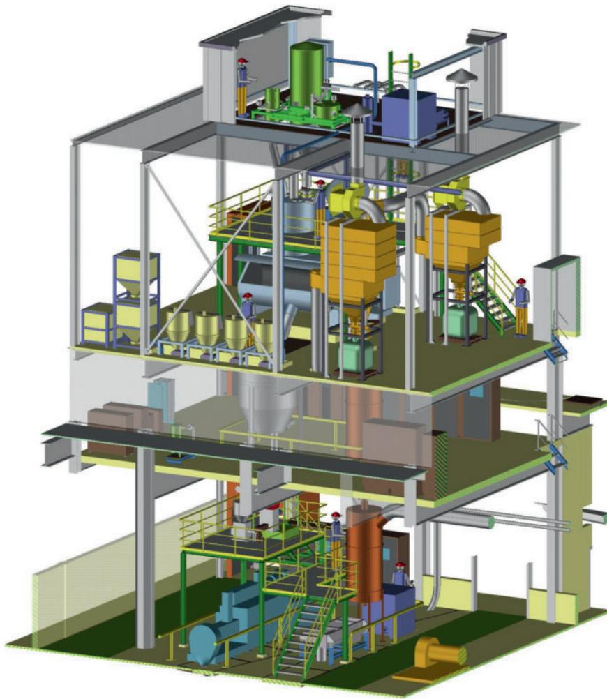
Emmen in the Netherlands. The system is over four stories high and achieves a throughput of up to 5,000 kg/h. The adapted kneading screw geometry allows eight formulations to be produced in rapid succession.
