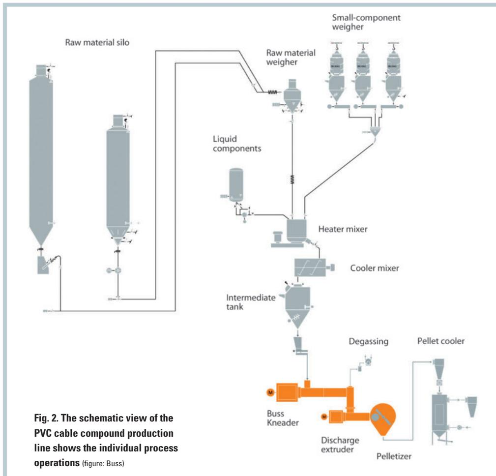
**Fig. 2. The schematic view of the PVC cable compound production line shows the individual process operations** (figure: Buss)
