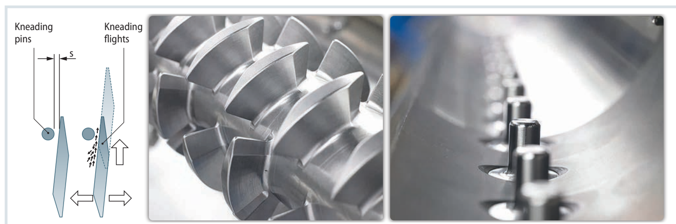
Fig. 3. In operation, the plastic mass is sheared in the shear gap (left) between the kneading flights (center) and kneading pins (right) [4]
